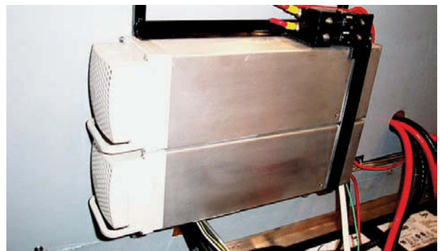
Figure 1 The vehicle uses two TDI Mercury battery-charging converters in series with the battery's center tap.
