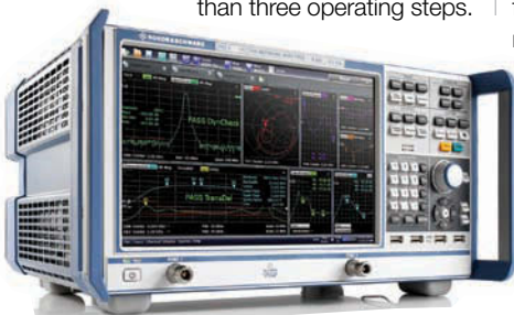
The ZNB and ZNC VNAs feature a dynamic range as high as 140 dB and a sweep time as low as 4 msec for 401 points.
